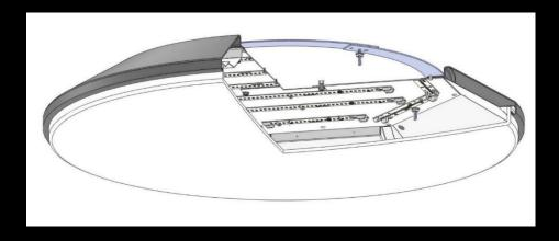
metal core LED boards mechanically held in place for simple field maintenance
